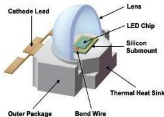
**Red LEDs** are based on aluminum gallium arsenide (AlGaAs). **Blue LEDs** are made from indium gallium nitride (InGaN). **Green LEDs** from aluminum gallium phosphide (AlGaP). "White" light is created by combining the light from red, green, and blue (RGB) LEDs. White - by coating a blue LED with yellow phosphor. Besides, an LED has:
