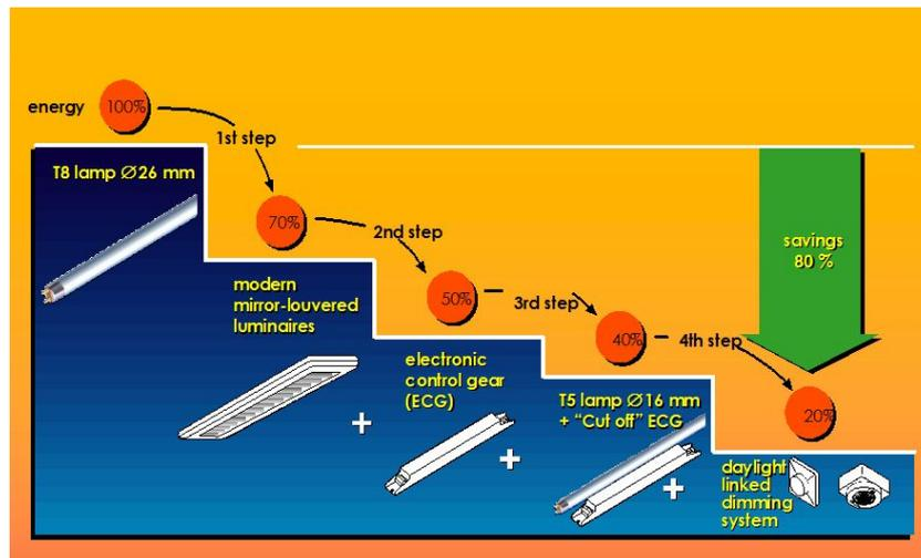
Fig. Energy saving by deploying dimmers
